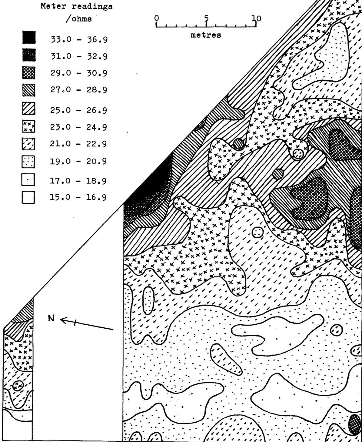
Readings were taken with the probes spaced 1 metre apart and along lines 2 metres apart.
